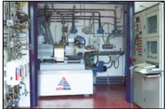
One of Three AESSEAL® Computer Controlled, 24hour test facilities which are used to qualify all of the companies API682 version 2 and ATEX product ranges.
