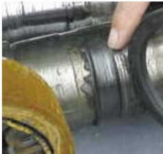
Shaft Damage from a Lip Seal
