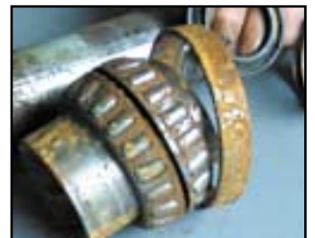
Moisture Contaminated Bearings.
